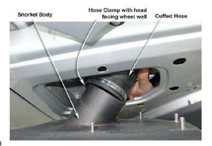
With the snorkel body correctly secured to the guard and upper mounting bracket, check the clearance of the snorkel body relative to the bonnet in the open and closed position, if required re-align the snorkel body of the guard to achieve adequate clearance.
